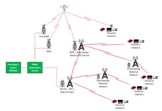
All EAS participants are required to monitor the assigned channels for inputs one (1) and two (2) on their EAS decoder. This action will enable relay of the national level emergency action notification (EAN) alert. The table that follows shows these recommended inputs. In addition, your local NWS station is also listed; it is recommended that it be tuned to input 3.
