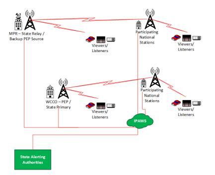
The secondary "legacy" method uses leased lines to send an audio message to the State Primary (SP) WCCO-AM and State Relay (SR) Minnesota Public Radio (MPR) as shown in the diagram below.
